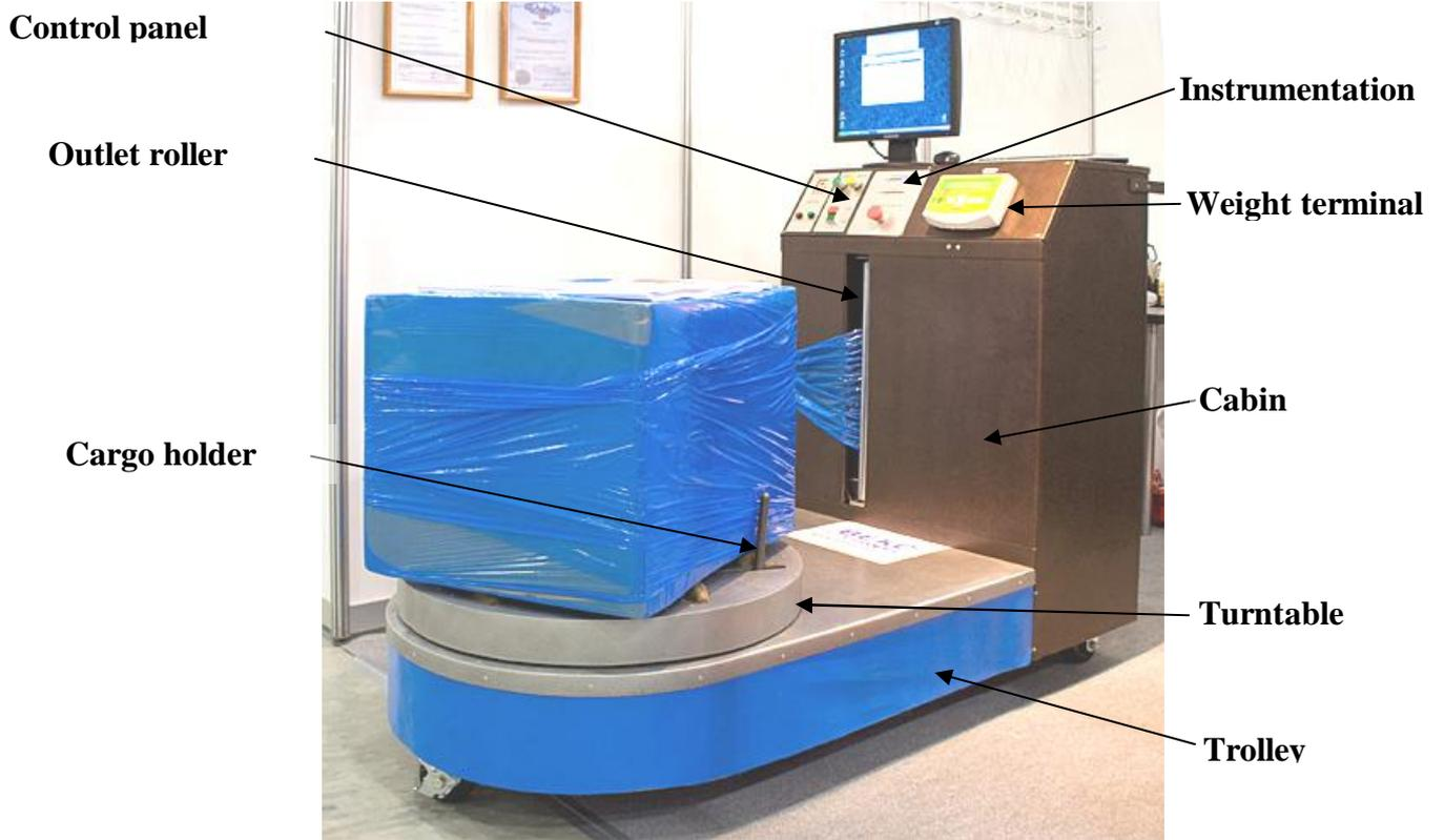
**Fig. 1. Packing Machine UPM-10V**
